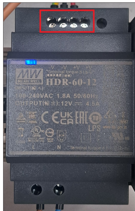
Fig. 1: Terminals to measure the output voltage
